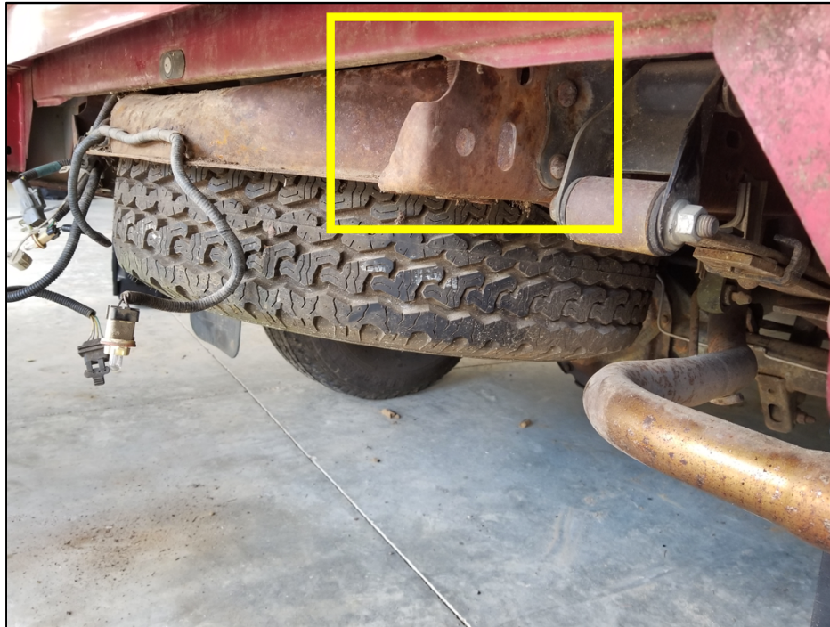
Figure 2. The primary attachment points to the frame are highlighted in this figure. This is an isometric view of the structure shown above.
